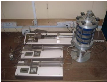
Computer controlled triaxial test for simulation of stress paths
