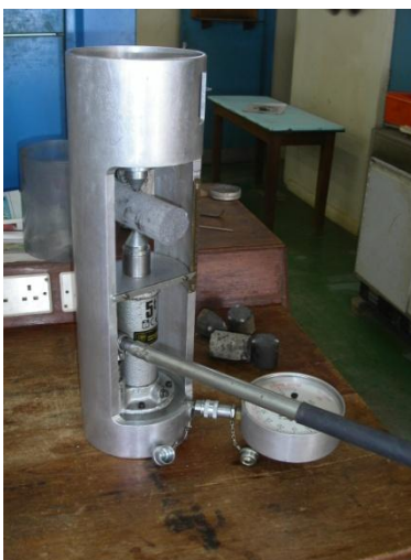
Point load index test for determination of compressive strength of rock cores
