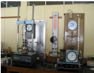
Triaxial test for determination of shear strength parameters with measurement of porewater pressures.
