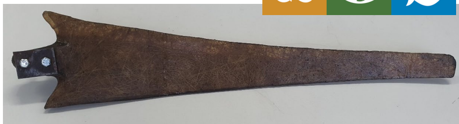
A 55 cm polyester-Pandanus utilis composite blade for a 0.5 kW wind turbine.
